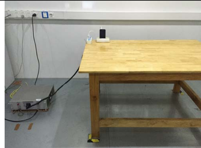
Conducted Emissions Test Setup Front View
