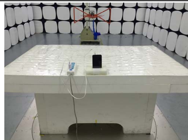
Conducted Emissions Test Setup Front View
