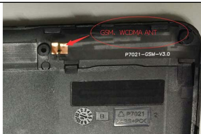
GSM/WCDMA Antenna View
