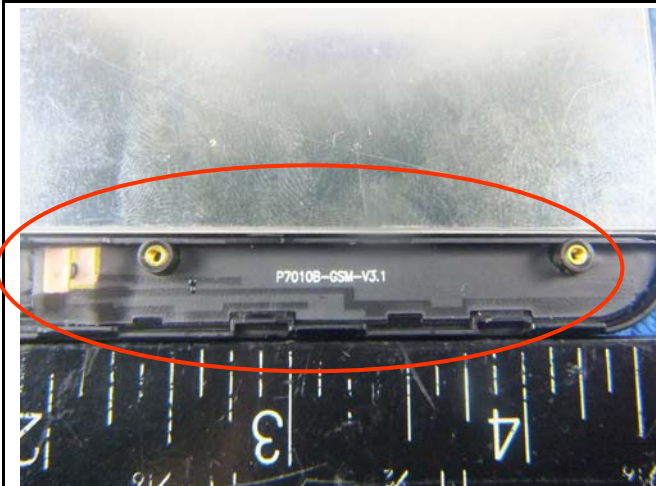
GSM/PCS/UMTS-FDD - Antenna View
