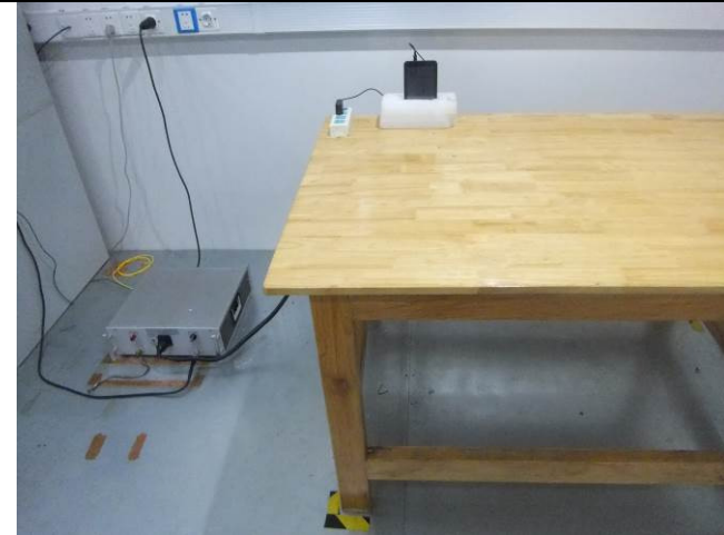
Conducted Emissions Test Setup Front View
