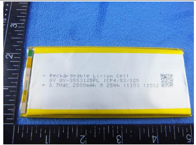
Battery - Front View
