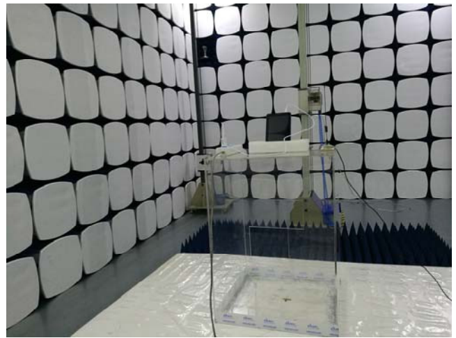
Radiated Spurious Emissions Test Setup Above 1GHz
