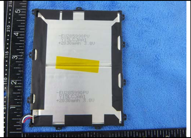
Battery - Front View
