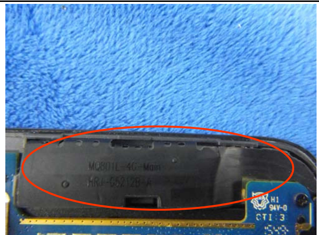
LTE - Antenna View
