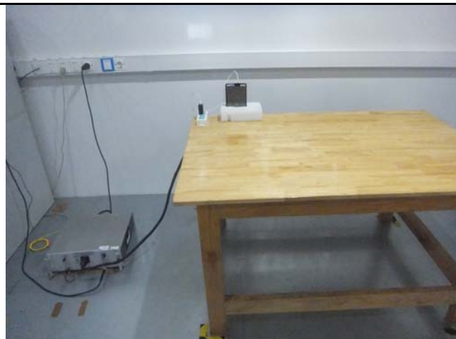
Conducted Emissions Test Setup Front View
