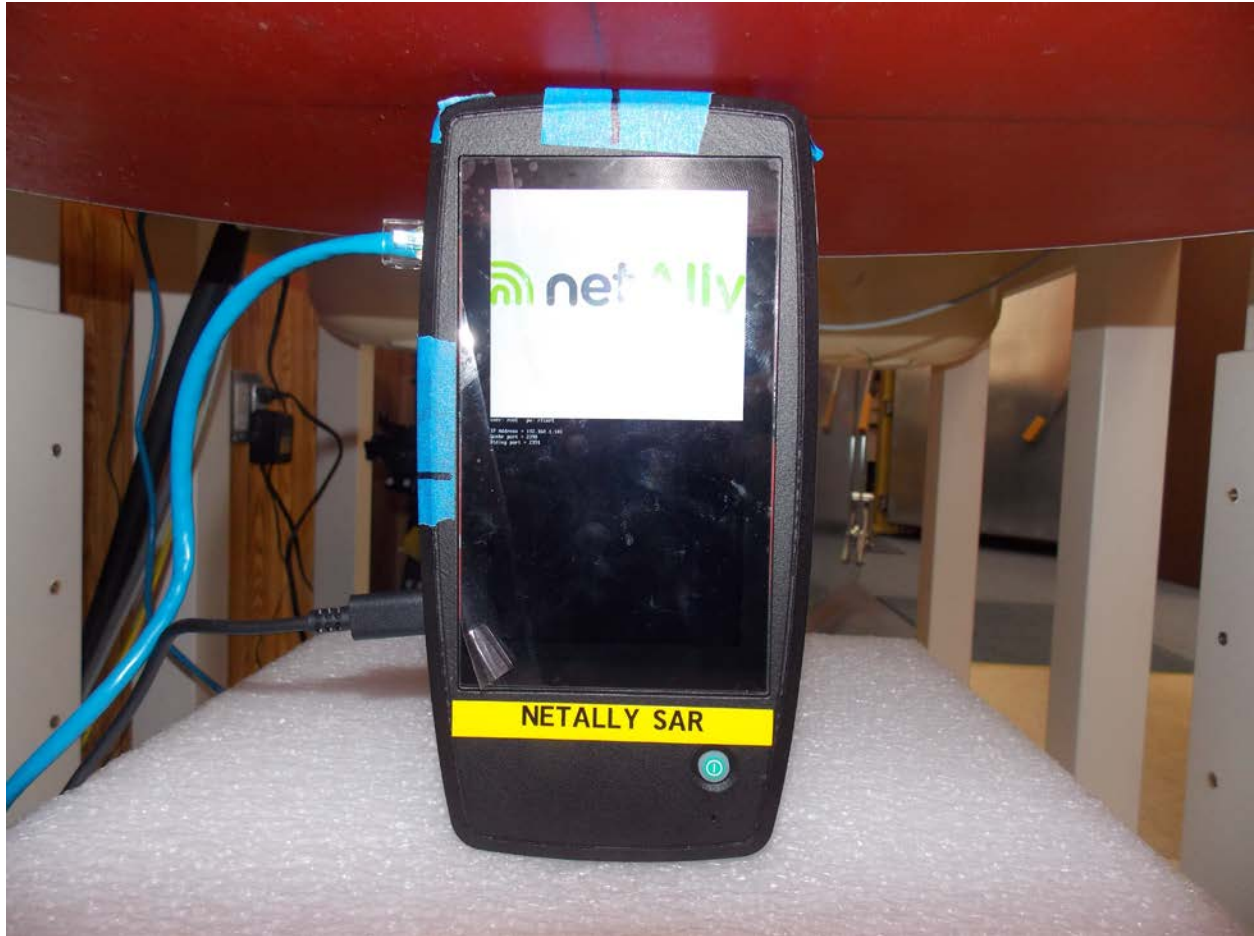
Test Position Top 0 mm Gap
