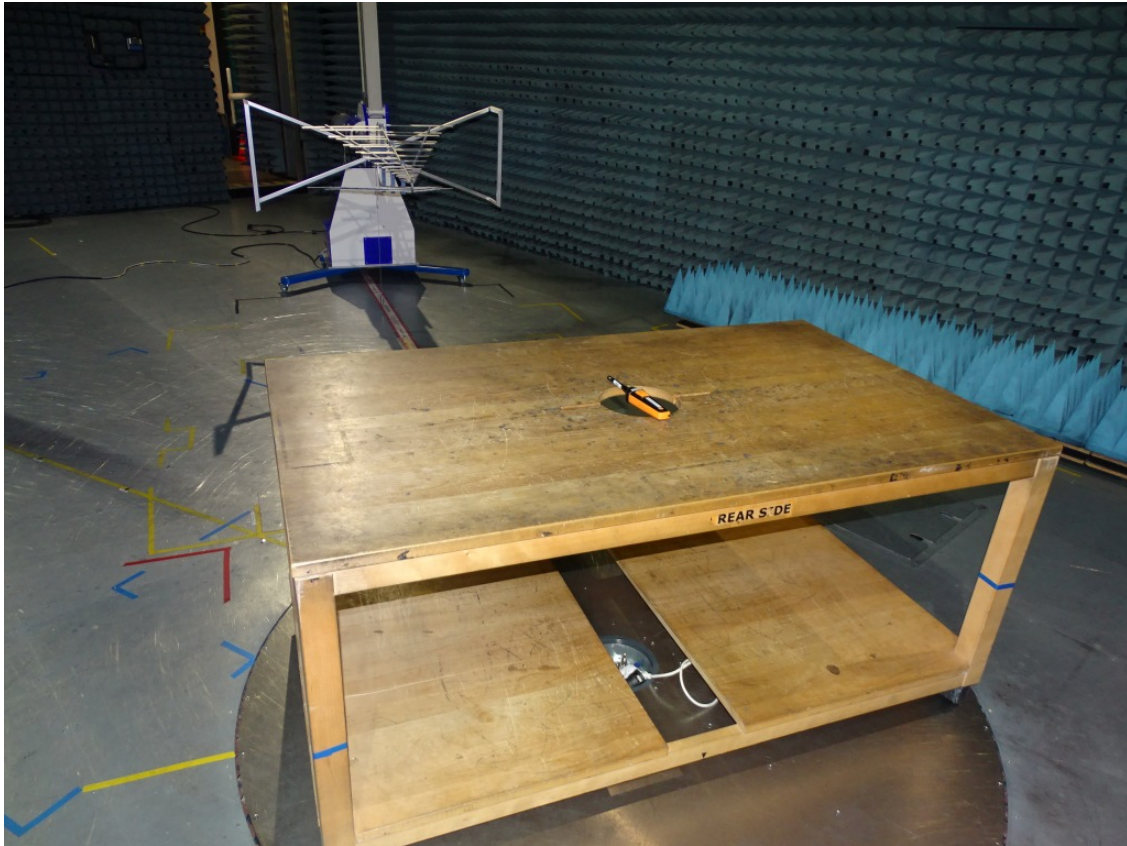
Photo 1: Test setup for radiated measurements (stand-alone, EUT supplied by a battery, unintentional radiator §15.109, ANSI C63.4) Below 1 GHz
