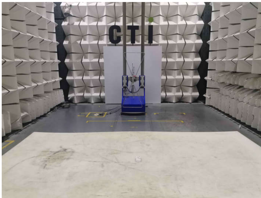
Radiated spurious emission Test Setup-1(Below 1GHz)
