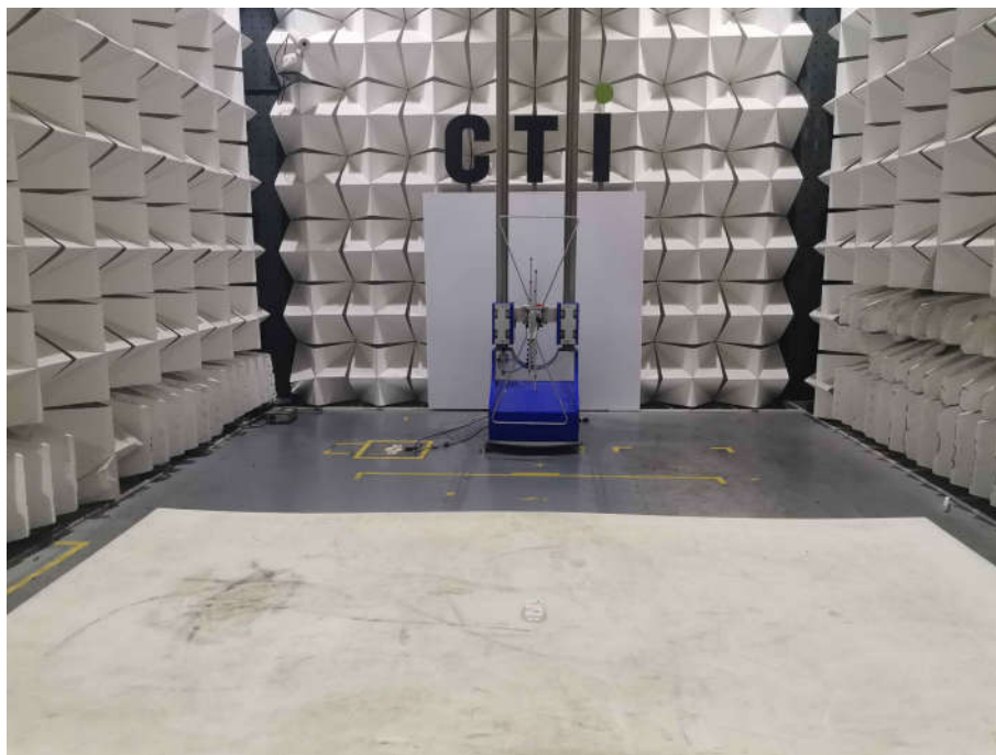
Radiated spurious emission Test Setup-1(Below 1GHz)
