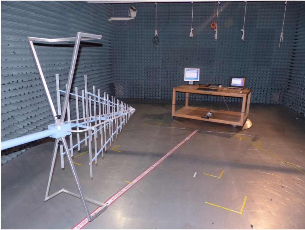
Photo 1: Test setup for radiated measurements (Enclosure, semi-anechoic chamber, 30 MHz to 1 GHz, unintentional radiator §15)
