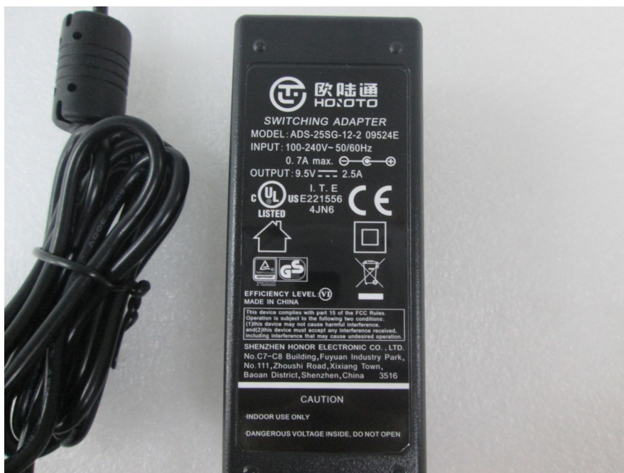
EUT – Adapter 1 Label View
