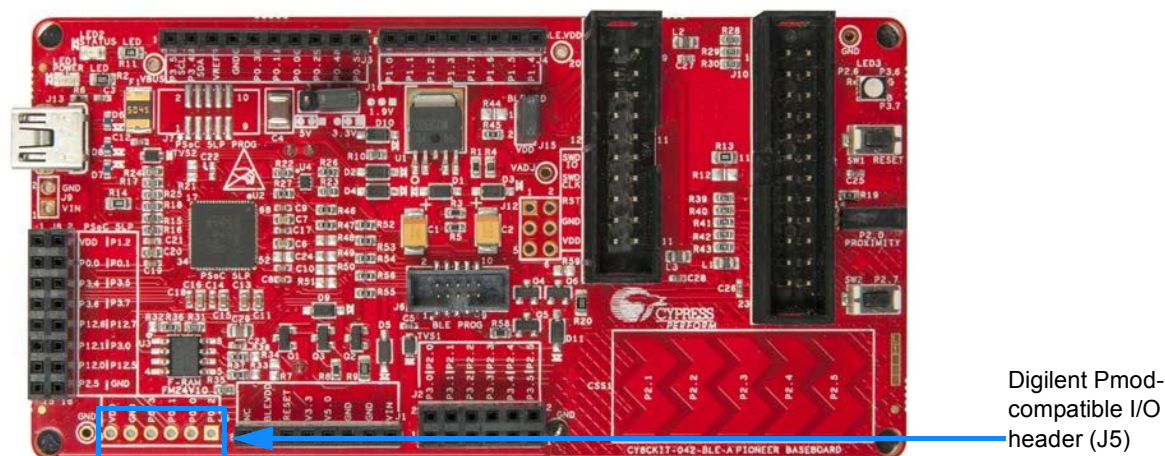
Figure 5-10. Schematics and Board Highlight of Pmod Connector
