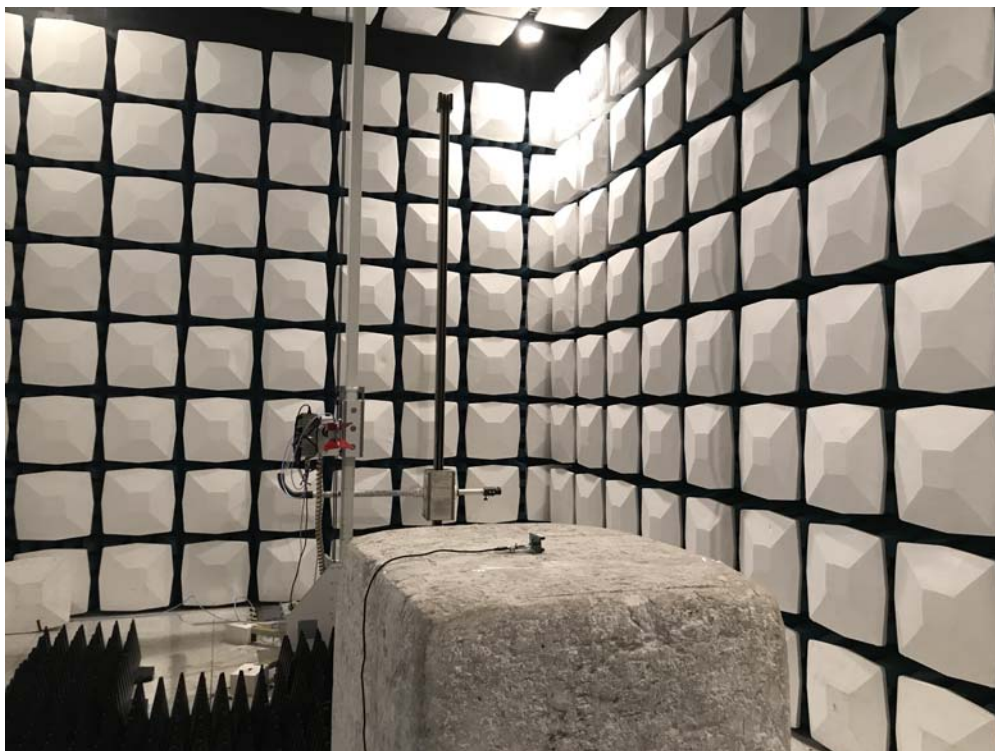
Description: Radiated Emission Test Setup for 1~18GHz
