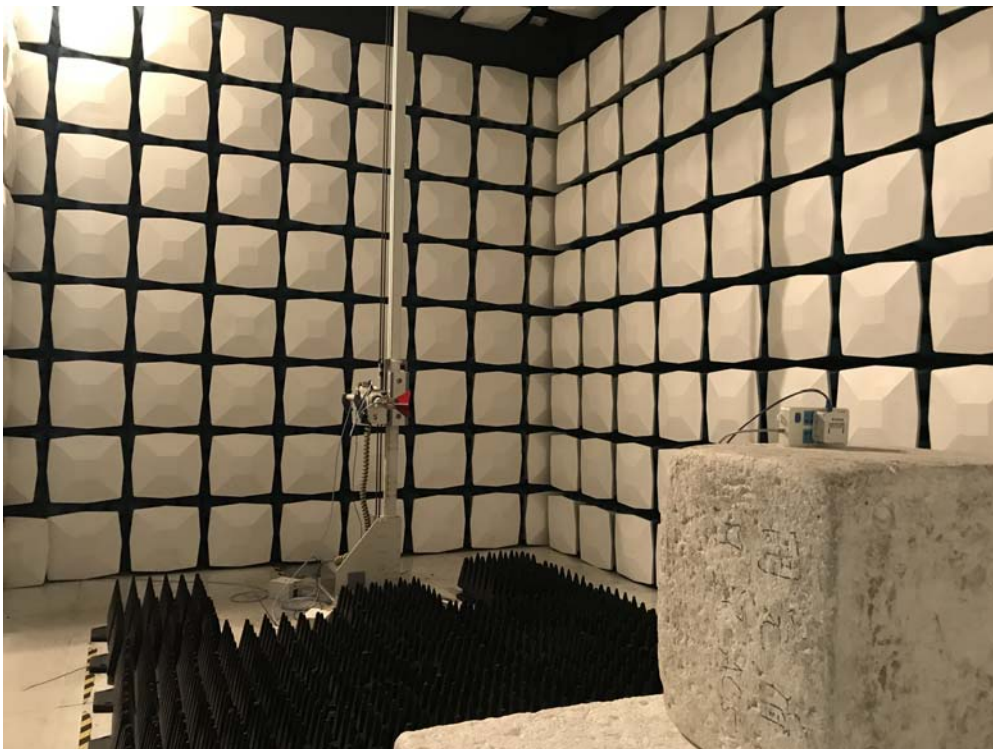
Description: Radiated Emission Test Setup for 1~18GHz
