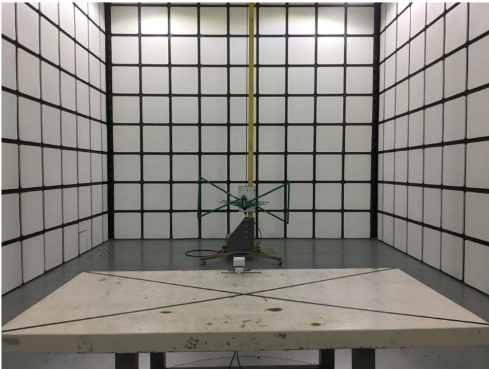
Description: Radiated Emission Test Setup for 1~18GHz
