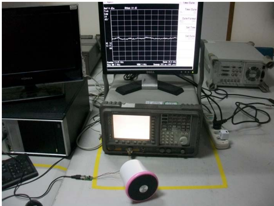
SPURIOUS EMISSION TEST SETUP
