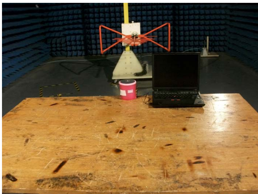
RE TEST SETUP
