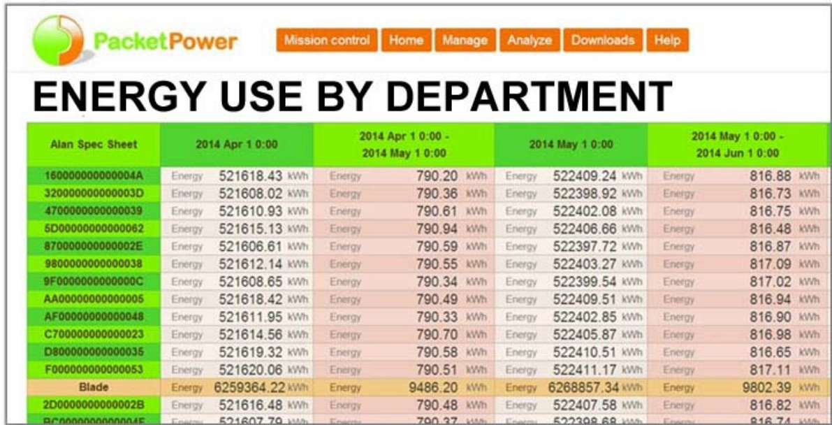
Figure 4: The EMX portal provides detailed energy use reporting and energy and power usage data along with alarm capabilities.
