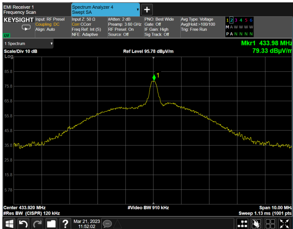
Plot # 1. Carrier frequency 433.92 MHz.
