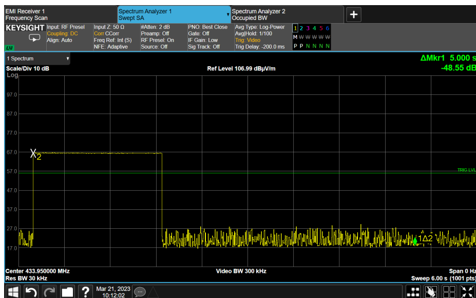
Plot # 8. Transmission within 5 seconds after activation
