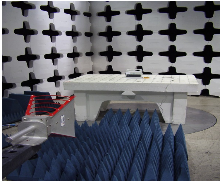
Photo 3. Radiated emissions test setup with Horn antenna.
