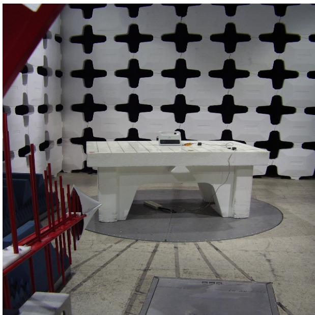
Photo 2. Radiated emissions test setup with Biconilog antenna.
