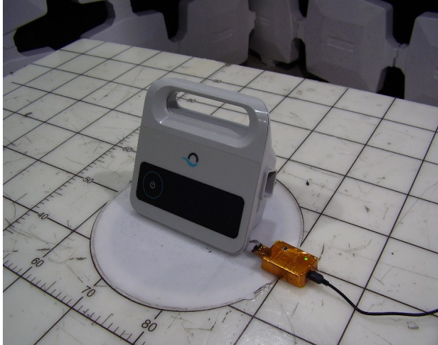
Photo 5. Radiated emissions test setup front view.
