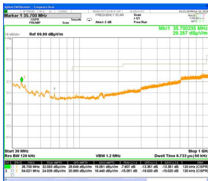
Plot # 27. Investigation result in 30 - 1000 MHz frequency range.
