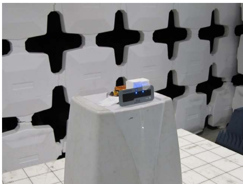
Photo 6. Radiated emissions test setup.
