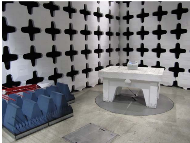
Photo 2. Radiated emissions test setup with Biconilog antenna.
