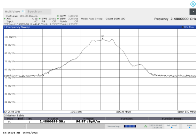
Plot 7.5.3 Peak spectral power density at high frequency for bitrate 1 Mbps
