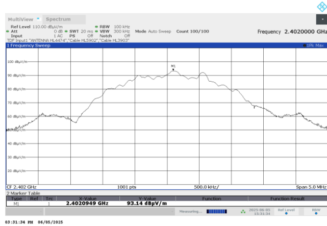
Plot 7.5.5 Peak spectral power density at mid frequency for bitrate 2 Mbps
