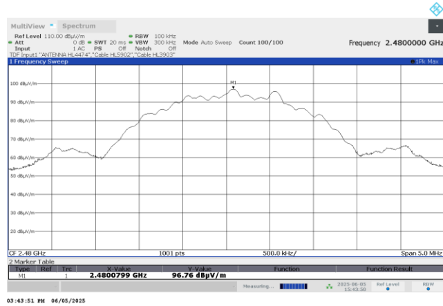
Plot 7.5.6 Peak spectral power density at high frequency for bitrate 2 Mbps
