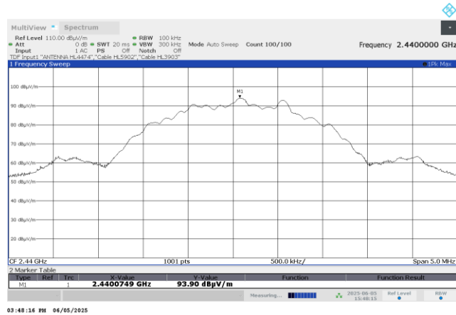
Plot 7.5.5 Peak spectral power density at mid frequency for bitrate 2 Mbps
