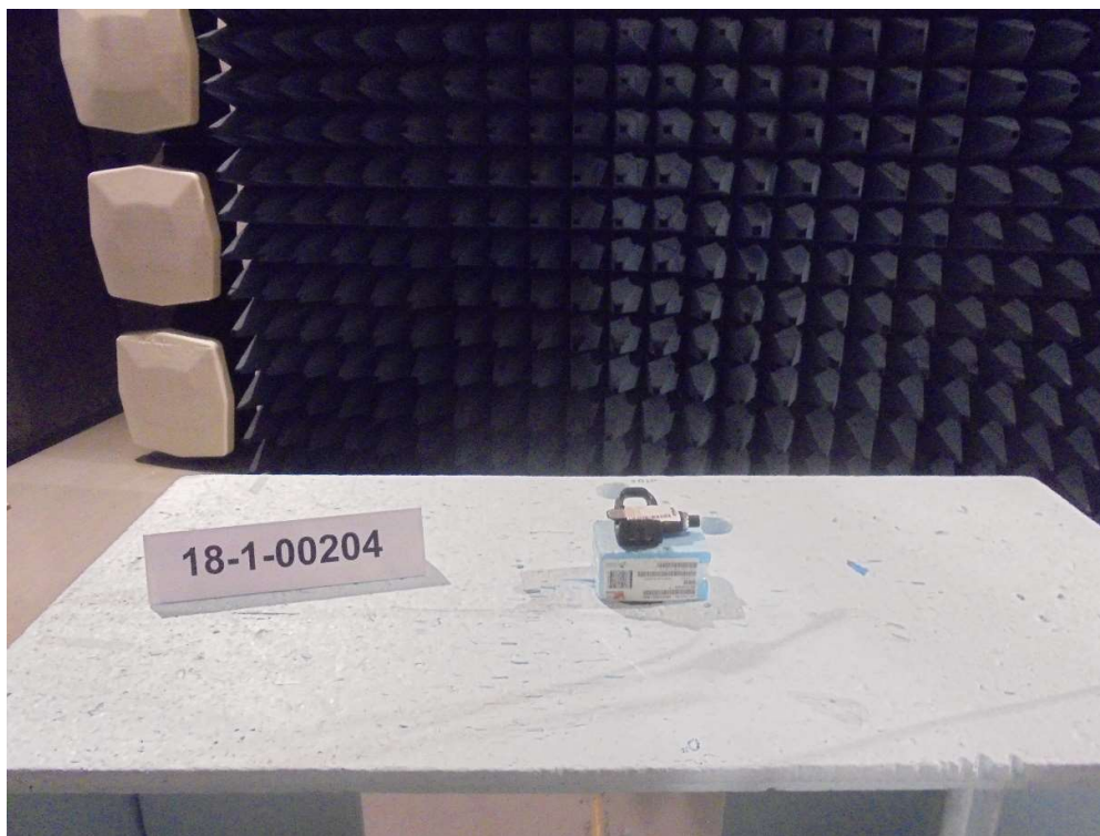
Photograph 1: Test set-up 3, EMI-field measurements
