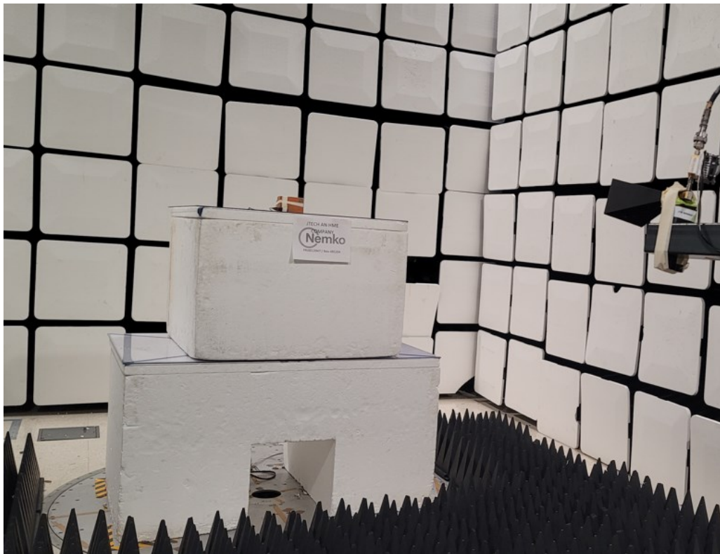
Figure 6 - Radiated emissions above 1 GHz (18 – 26 GHz), front view.
