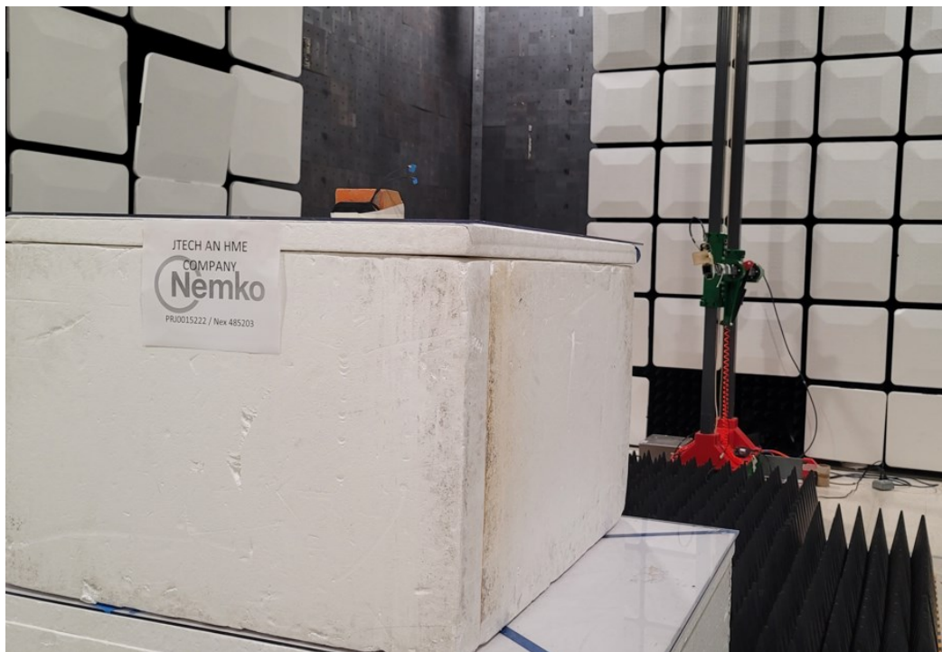
Figure 7 - Radiated emissions above 1 GHz (18 – 26 GHz).
