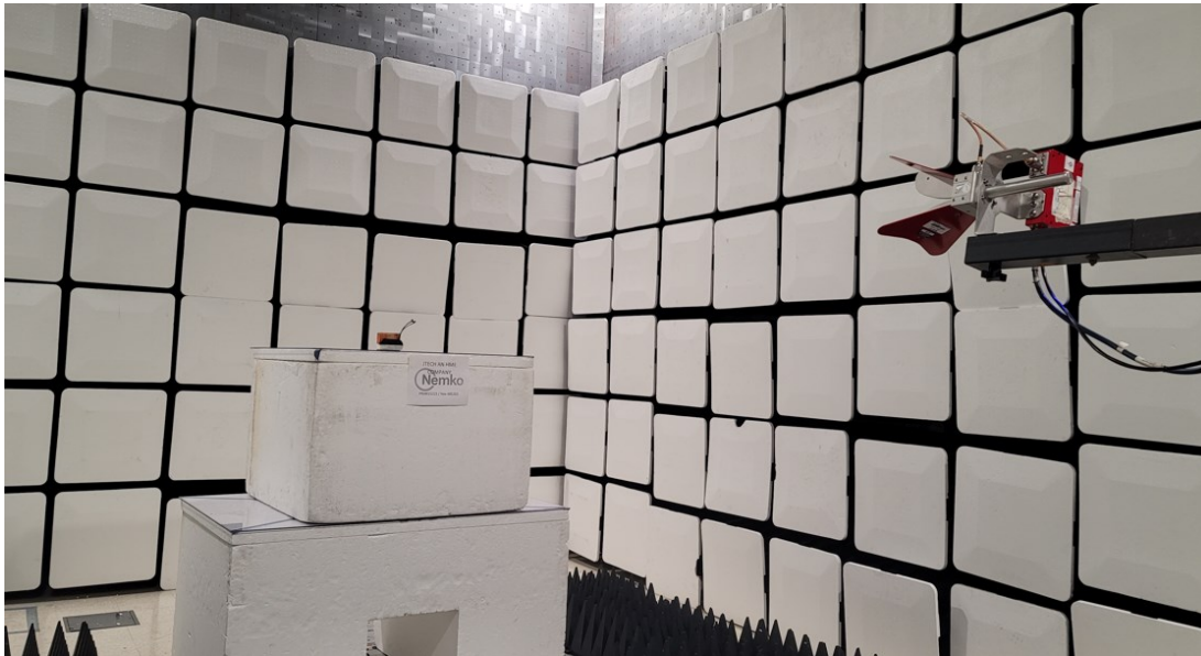
Figure 4 - Radiated emissions above 1 GHz (1 – 18 GHz), front view.
