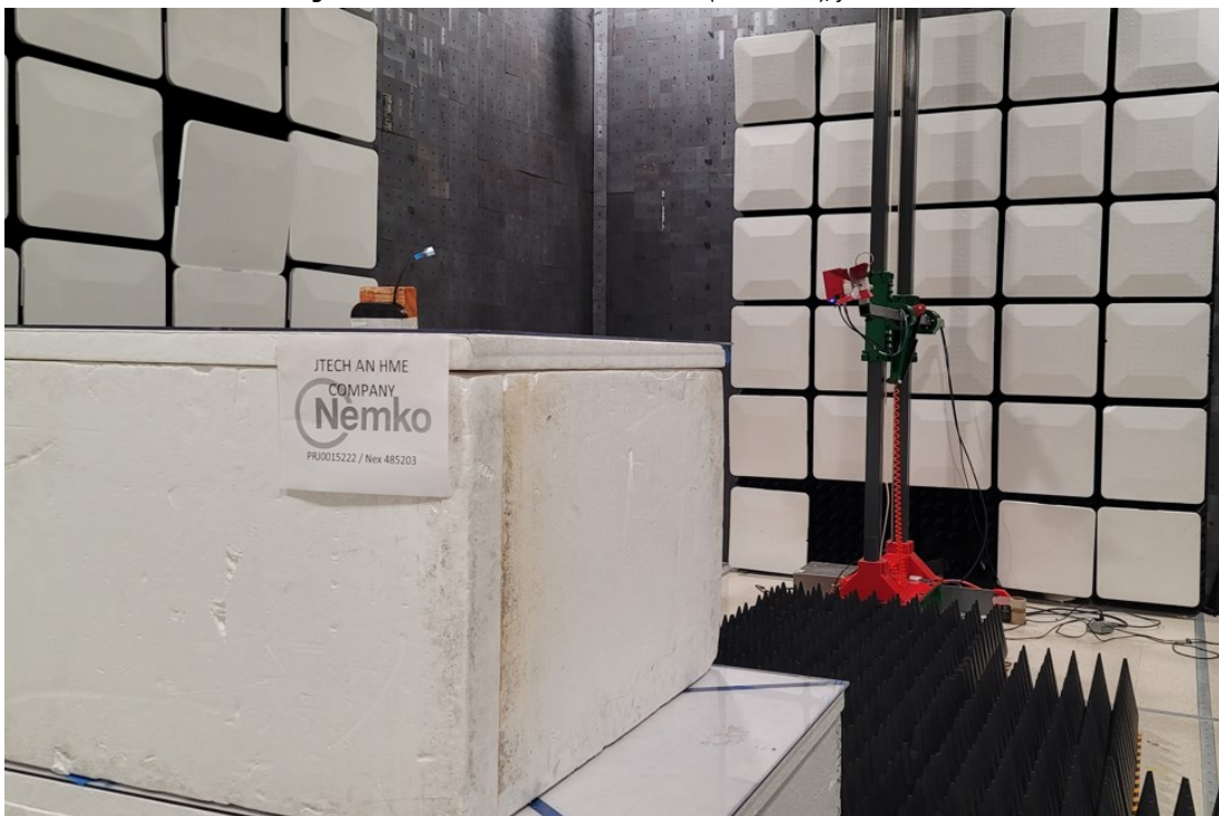
Figure 5 - Radiated emissions above 1 GHz (1 – 18 GHz), rear view.
