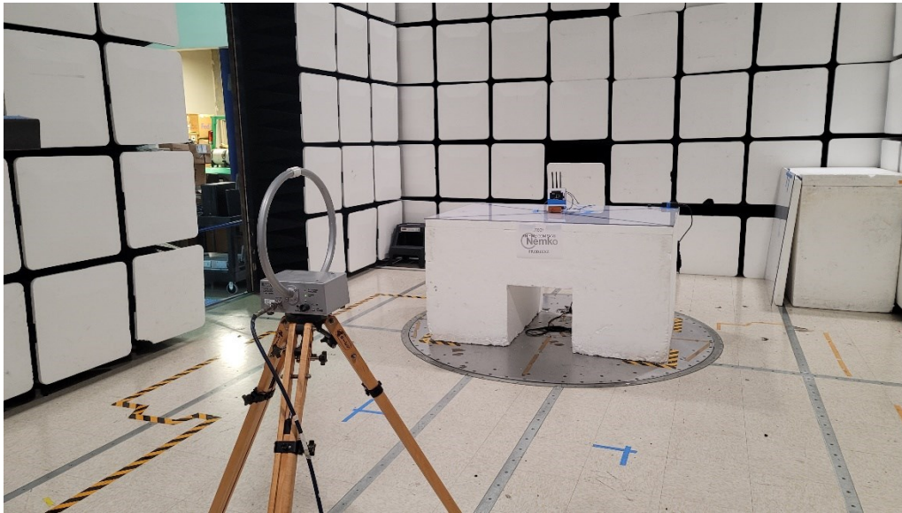
Figure 4 - Radiated emissions below 30 MHz (9 kHz – 30 MHz), 90 Degrees, front view
