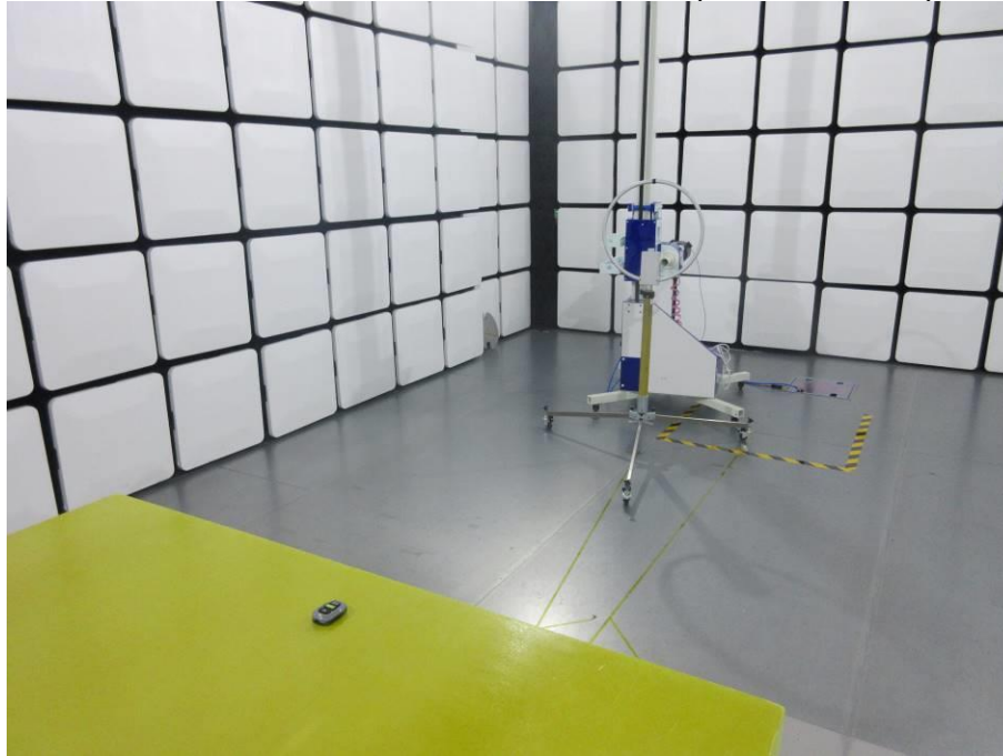
RADIATED RF MEASUREMENT SETUP (9kHz ~ 30 MHz)
