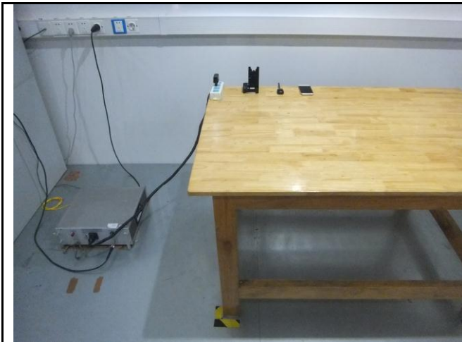
Conducted Emissions Test Setup Front View
