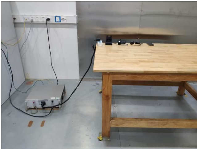
Conducted Emissions Test Setup View
