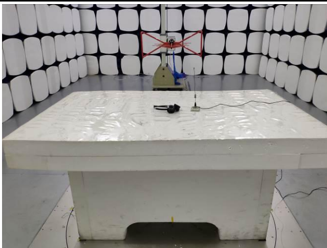
Radiated Spurious Emissions Test Setup Below 1GHz
