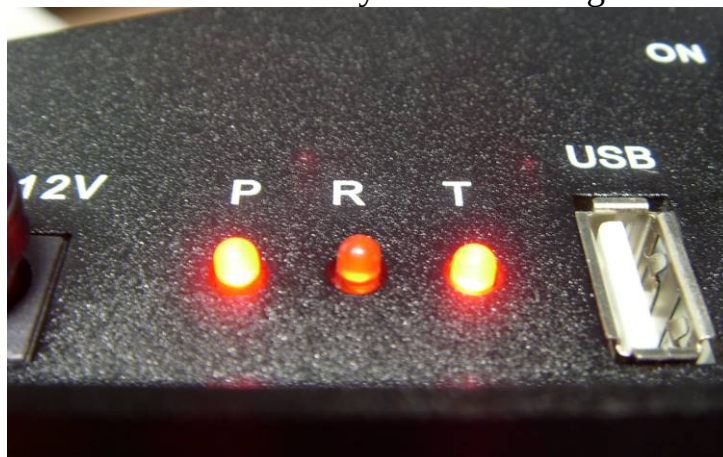
Picture for CA into transmitting status
