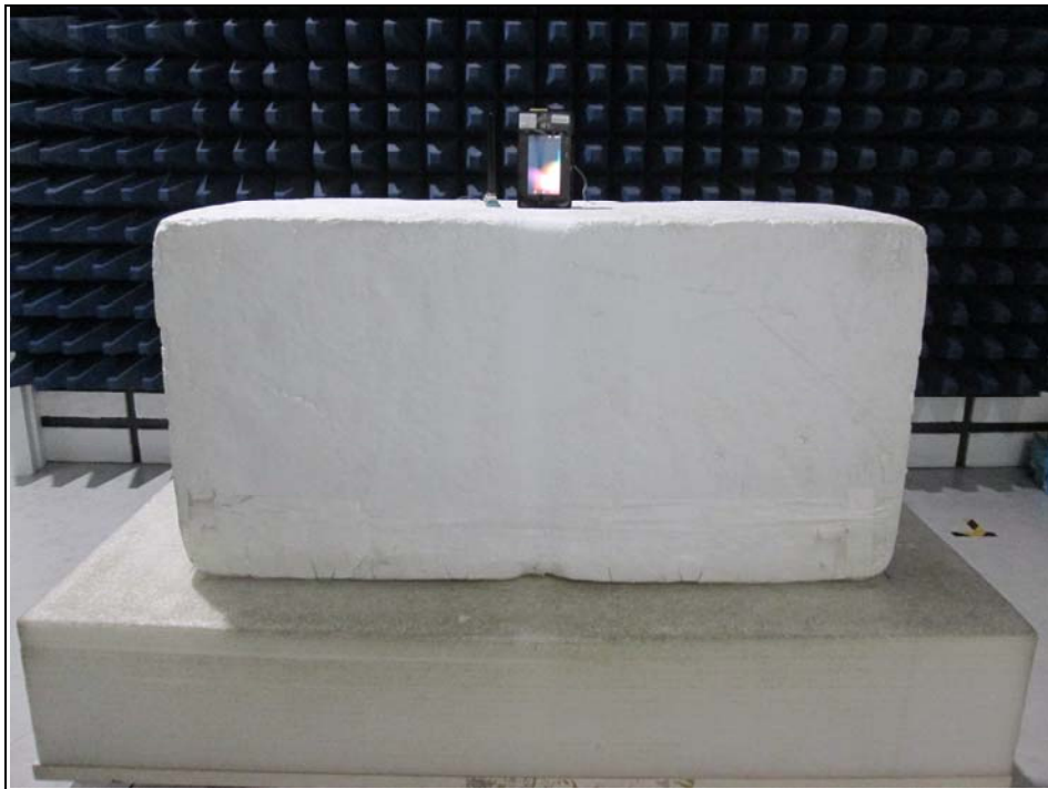
Radiated Emission above 1GHz Test
