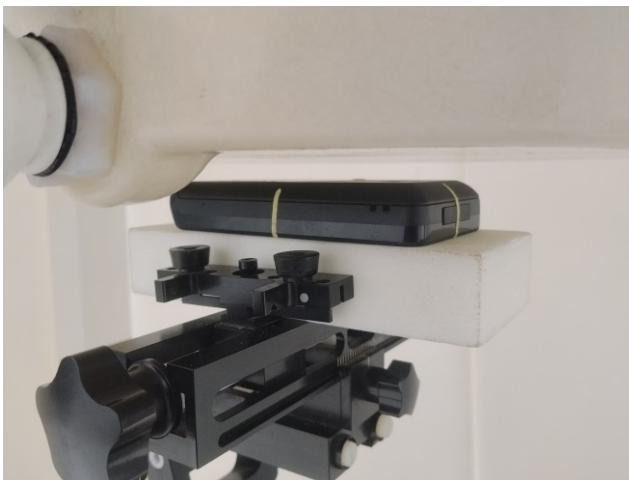
Back, Test Separation 10 mm
