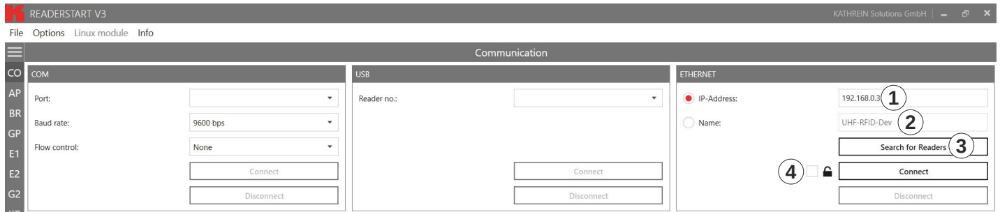
Fig. 14: Establishing connection to the reader
