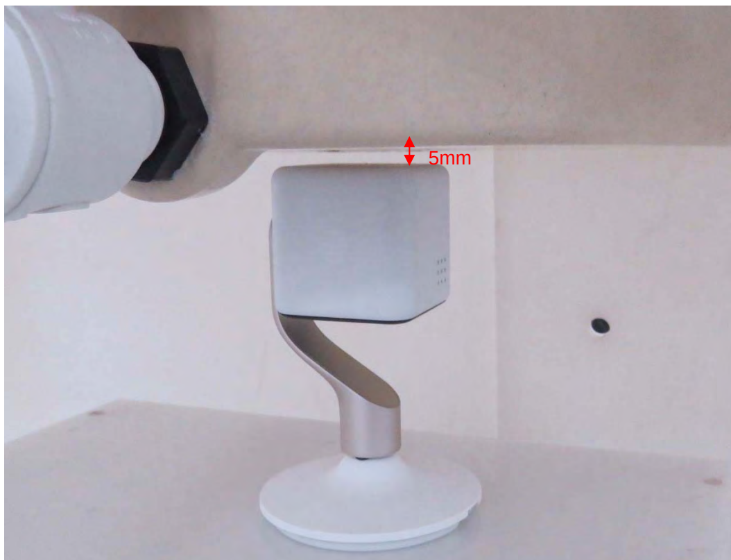
Picture 8: Back Side, the distance from EUT to the bottom of the Phantom is 5mm
