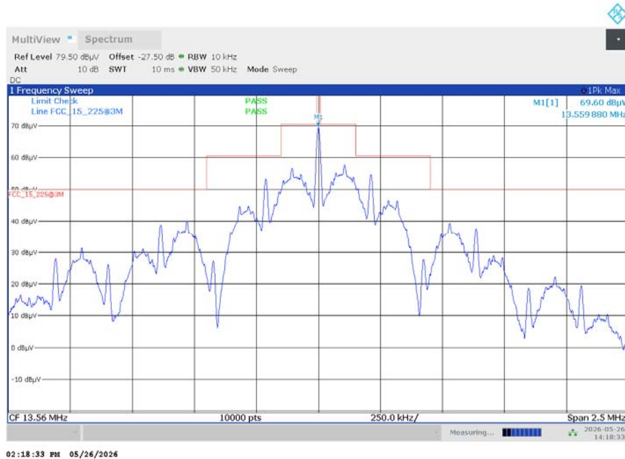
Plot 3: Spectrum mask (the limits are recalculated according to the ANSI C63.10-2013 sub clause 6.4)
