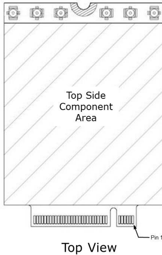
Figure 10 RF Antenna – Coaxial Connector Location
