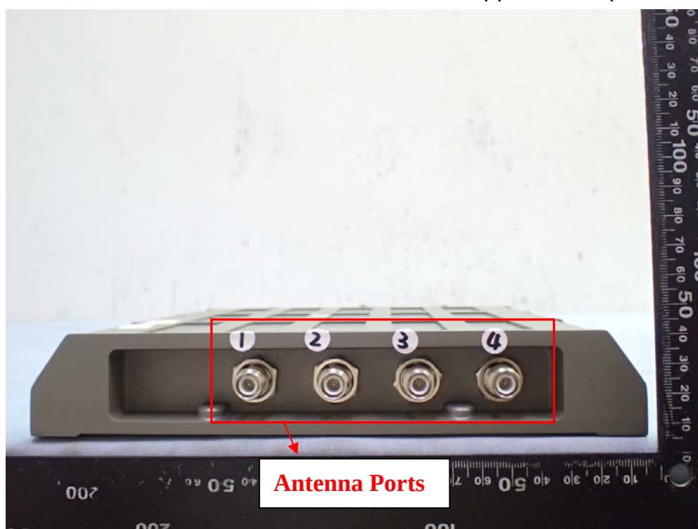
Figure 3 General Appearance (Antenna Ports)
