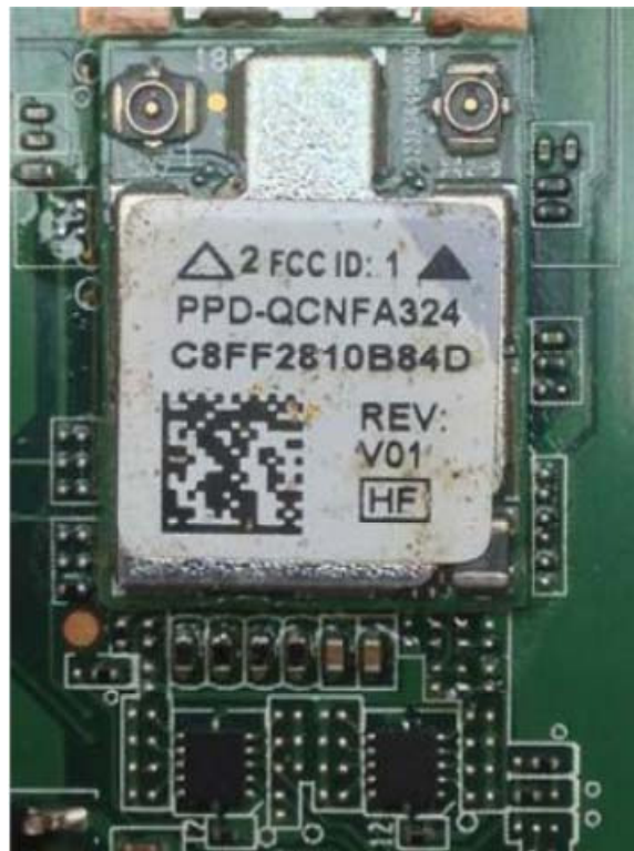
Figure 36 7" Multi Function Pad, Internal View (Wireless Module)
