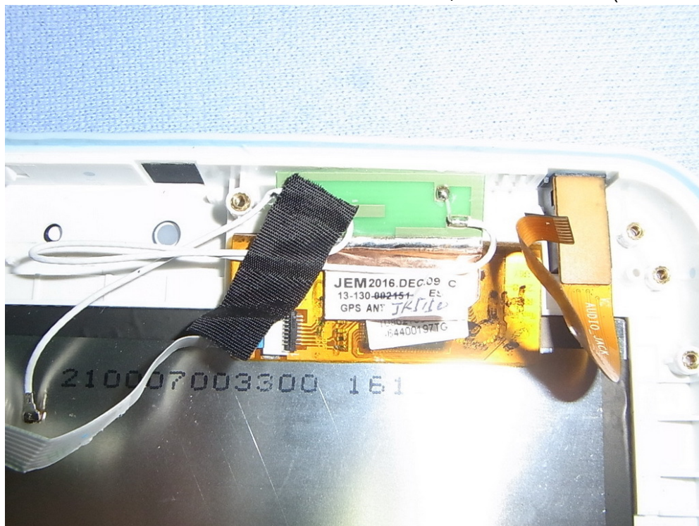
Figure 46 7" Multi Function Pad, Internal View (GPS Antenna)
