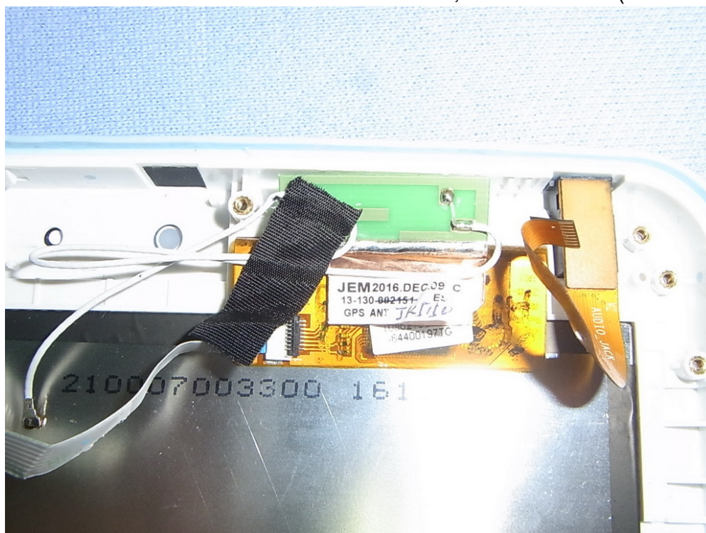
Figure 46 7" Multi Function Pad, Internal View (GPS Antenna)
