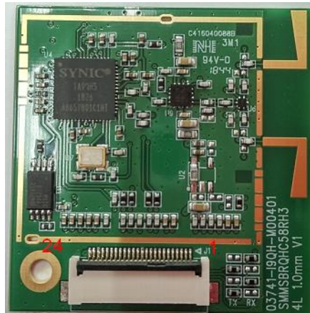
Fig 8.1 Pin sequence of SY5-A24-F Module
