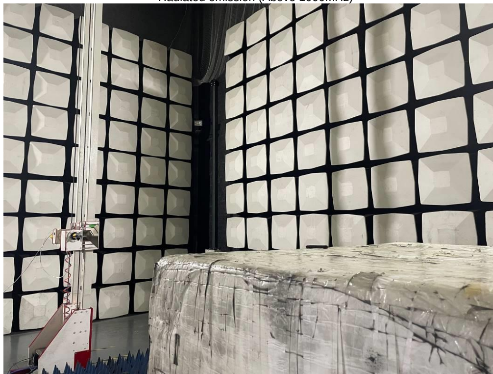
Radiated emission (Above 1000MHz)
