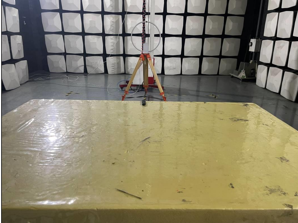
Test Photo Radiated emission (Below 30MHz)
