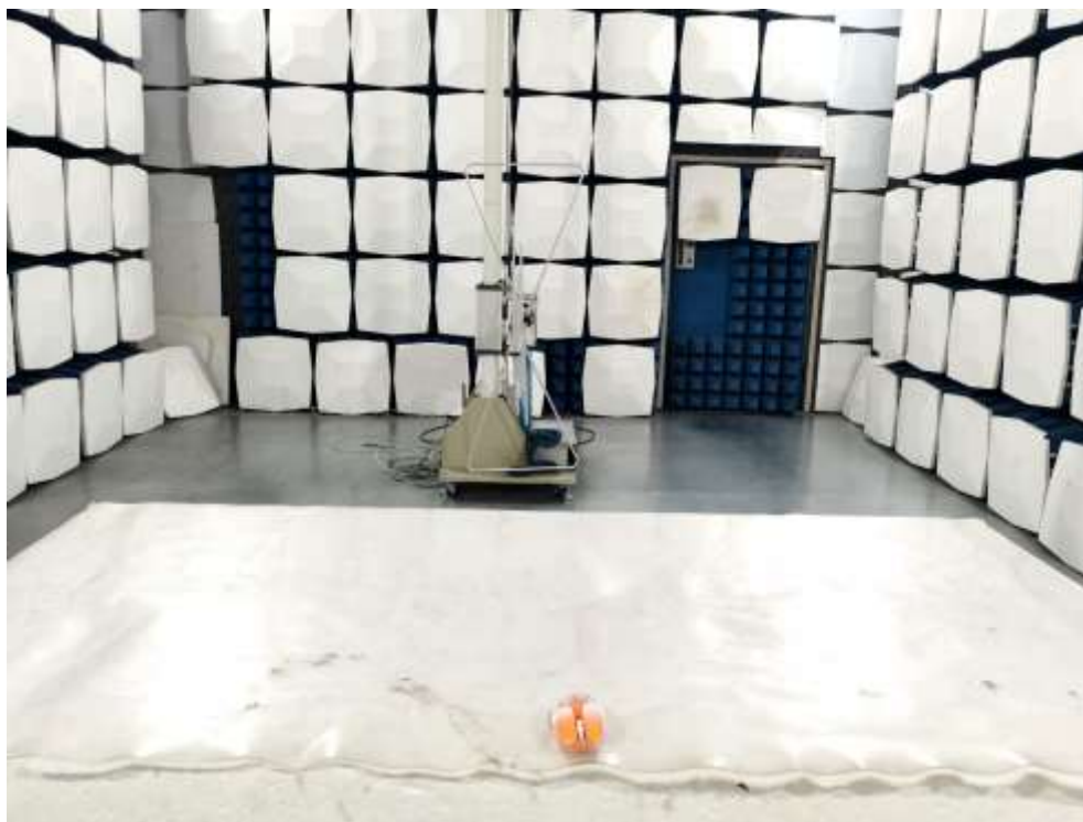
Radiated Emission Test Setup:
