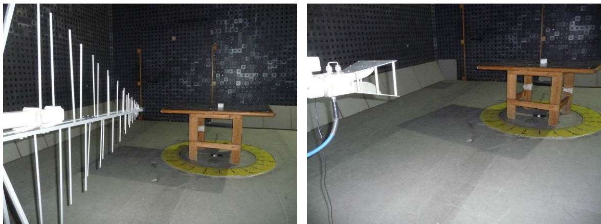
Photograph 7.7.1 Setup for radiated emission measurements
