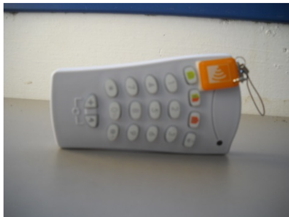
Photograph 6.4.2 EUT in Y-axis orthogonal position
