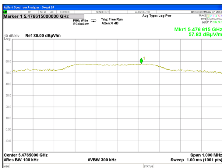
Plot 7.7.32 Radiated emission measurements at the sixth harmonic of mid carrier frequency
