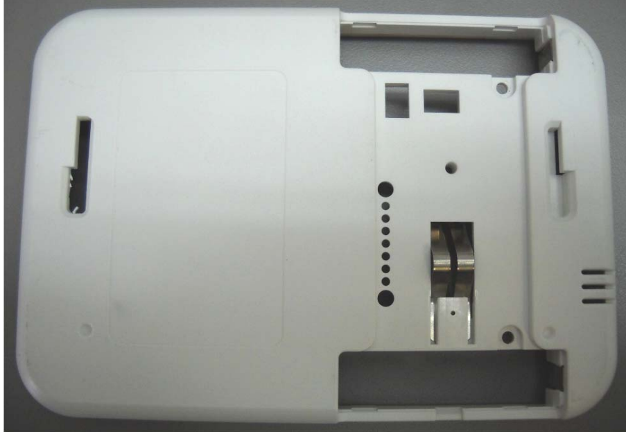
Photograph No.3 Touch screen keyprox rear side view with cover removed
