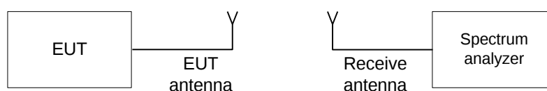
Figure 7.1.1 The 20 dB bandwidth test setup
