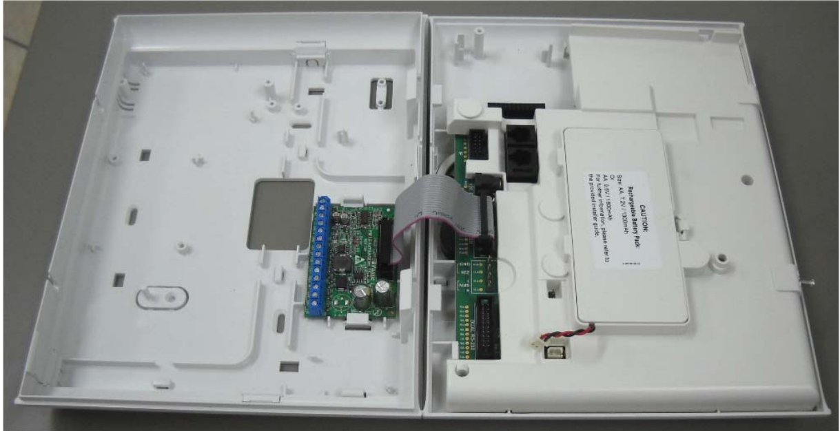
Photograph No.1 PMASTER-30 control panel internal view
