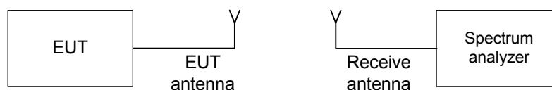
Figure 7.3.1 Occupied bandwidth test setup
